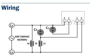
Model Name ECS224L Operating voltage AC 220V, 50/60Hz Application CSIR or CSCR Motors (0.18~3.7kW)
