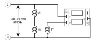
M1/M2: Main coil, ST: Auxiliary coil
